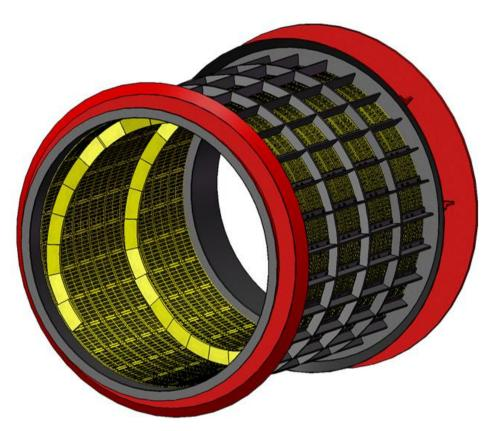
Besides the utilisation of our *Lock-out* pins and sleeves allow the operator to effect both de-installation and installation procedures inside the mill without the need of any colleague supporting him from outside.
