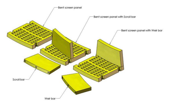
The Trommel screen panels are custom bent so to perfectly fit the screen frame. Weir bars and Scroll bars are available on request so to help the screening efficiency.
