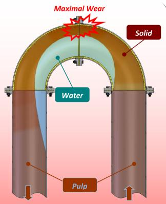
When flowing into the elbow the solid part of the pulp gets separated from the liquid part because of the centrifugal force.
