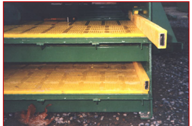
5. Install lateral bars
